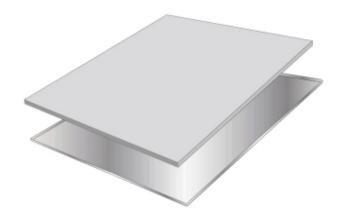
Steel Tray Paver Support are made of galvanized steel sheets with downturned edges of 3/8" on the four sides, they are double folded to empower the underside of the 3/4" thick pavers and grant them an extra strength.
